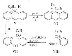
less crystalline compound having the composition expected for 2-(2-picolinyl)-benzophenone (VII). This structure was suggested further by the infrared absorption spectrum which showed the presence of the carbonyl group, but indicated that carboxyl was absent. The new diketone (VI) was synthesized from o-benzylbenzonitrile (VIII) by reaction with o-pyridyllithium followed by oxidation. This demonstrates beyond any doubt that phenylmagnesium bromide attacks the acridizinium nucleus at position 6.
